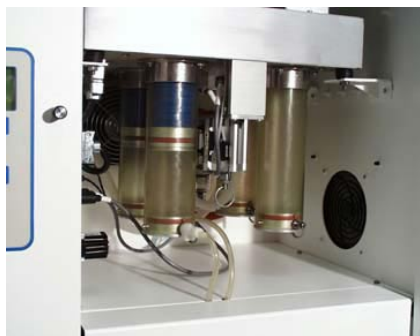
Partisol plus – Filters for PM 10 compartment
